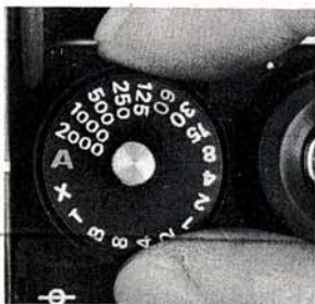
Setting shutter-speed dial at "A" position or marked speeds is quite similar to that on other auto-exposure Nikon cameras such as FE, EL2. To prevent accidental movement from "A" setting, you must push central hub to turn to manual speeds
