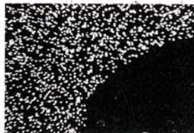
You can't see oval holes in F3's main mirror by just looking, but this backlit photomicrograph reveals part of the random, keyhole-shaped pattern.
