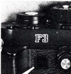
Ten-sec. blinking electronic self-timer LED is welcome, but can't be seen when motor is attached to camera.
