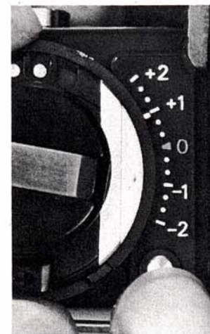
Auto-exposure-compensation dial is calibrated in 1/3 stops, has range of ± 2 f/stops with locking mechanism at each marked setting.
