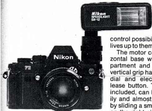
SB-12 Nikon flash unit fits securely on F3, but must be removed in order to rewind film manually.
