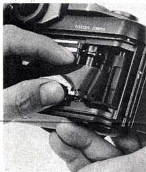
One of few plastic parts in camera, multi-slotted take-up spool seems great improvement over Nikon's former ones.
