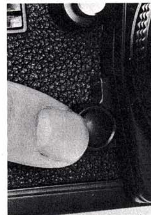
Exposure memory lock button allows close-up metering to be done on auto exposure and also holds exposure indication in finder. It's handy, but not when motor drive is attached.
