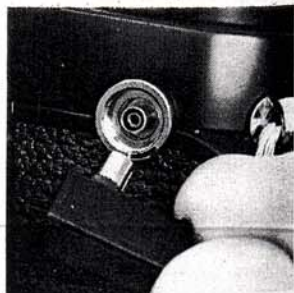
Threaded PC terminal allows all PC-connected flash units to be attached to Nikon F3 but, if you use this terminal, you do lose the advantages of Nikon's own dedicated automatic flash.
