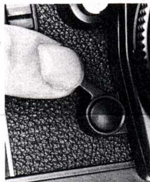
Batteries and/or electronic give out? You can still use F3 with mechanical shutter-release lever at 1/60 sec.
