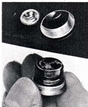
Two 1.5-volt silver oxide batteries in bottom clip usually power camera, but motor's own power takes over whenever MD-4 motor's attached.
