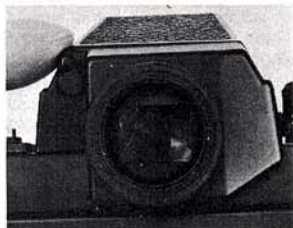
Eyepiece shutter lever at rear of prism prevents extraneous light from entering viewfinder during automatic exposures when your eye is not right up to eyepiece window.
