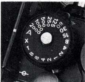
Self-timer turn-on lever is quite similar to that of meter turn-on lever adjacent to it and can be mistaken for it by those not thoroughly familiar with the camera.
