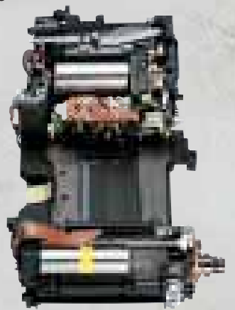
Rear chassis — film rewind and shutter charge mechanism
