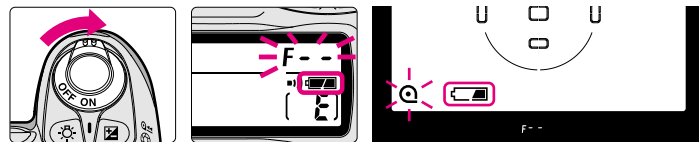
Sufficient battery power
